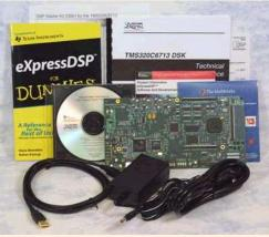
The DSK features the TMS320C6713 DSP, a 225 MHz device delivering up to 1800 million instructions per second (MIPs) and 1350 MFLOPS. This DSP generation is designed for applications that require high precision accuracy. The C6713 is based on the TMS320C6000 DSP platform designed to needs of high-performing high-precision applications such as proaudio, medical and diagnostic. Other hardware features of
